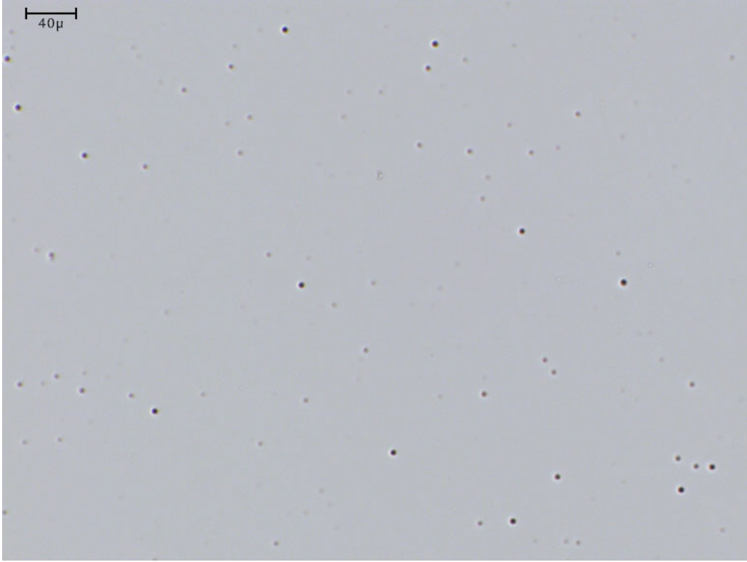
Figure 2.6: Microscopic image of an irradiated and etched SSNTD of a tissue standard with 10ppm of boron.
