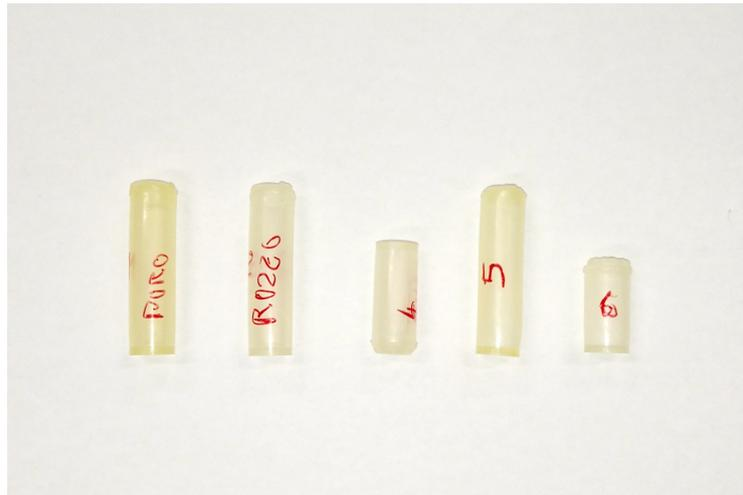
Figure 2.1: Irradiated samples of aluminum fluoride powders
