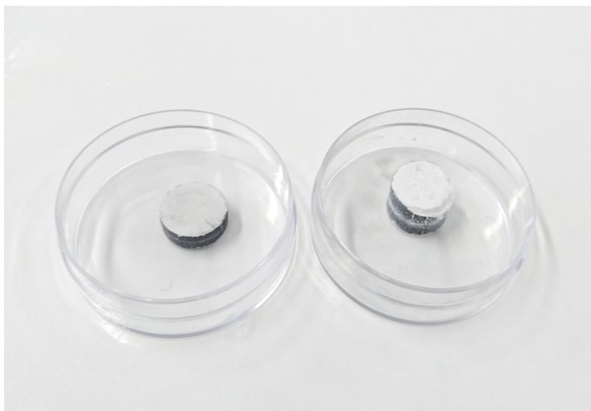
Figure 2.19: Samples of sintered  $AlF_3$  after an irradiation of 20 hours
