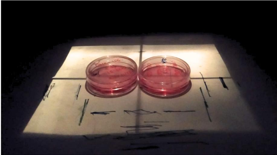
Figure 4.2: The Petri dishes with the UMR106 cells before the irradiation, placed below the X-ray Tube, November 2022, Naples.
