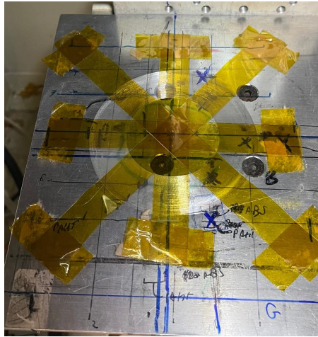
Figure 3.9: Photograph of the 20 m P-doped silica fiber arranged in a monolayer coil of 2.5 cm radius for irradiation.
