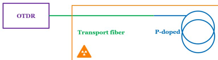
Figure 3.8: Schematic layout of the RIA experimental setup. A single-mode P-doped fiber was spooled in a monolayer geometry and interrogated with the OTDR during irradiation. A radiation-hard transport fiber was used to connect the exposed section to the instrument, ensuring that the measured attenuation variations originated solely from the irradiated sample.
