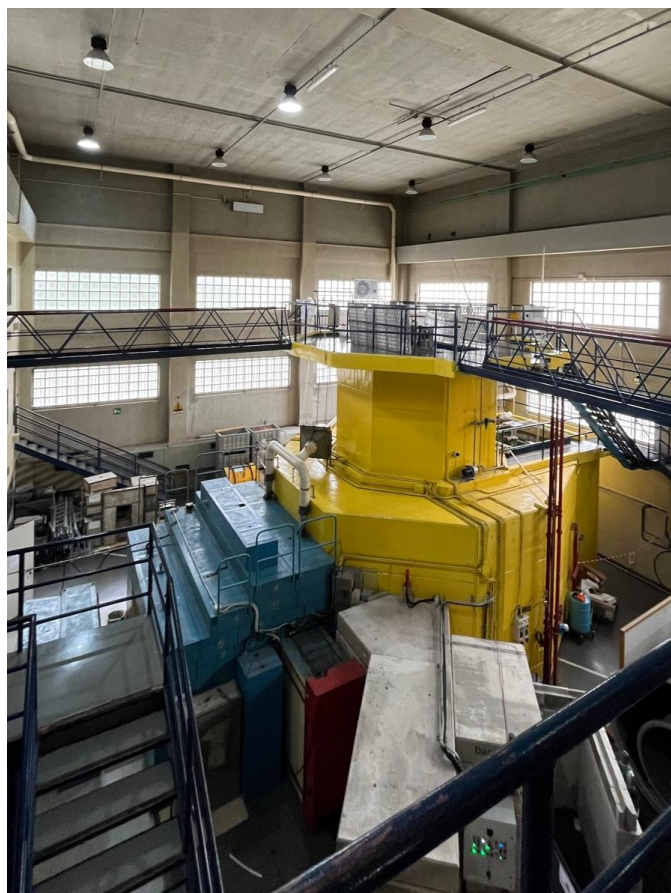
Figure 2.1: Picture of the TRIGA Mark II reactor of the University of Pavia, Italy. The yellow part of the reactor is the core, while the Thermal Column is visible in blue. The gray block is the thermalized channel.
