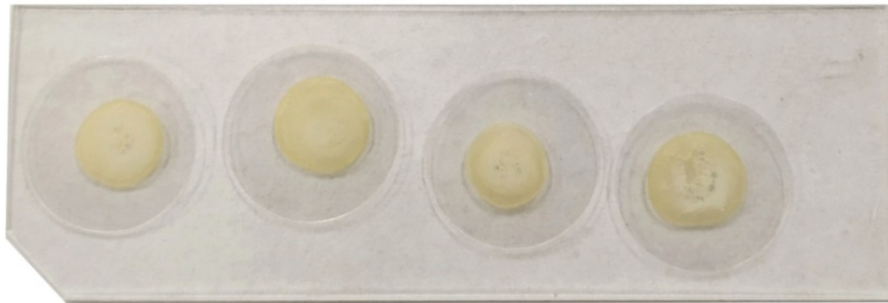
Figure 2.4: Solid sample positioned on a CR-39. For proper reference, the samples are numbered starting from the cut at the top right corner when the CR-39 is vertical.
