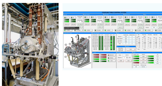
Fig. 2 - The radiation hard ISOL front-end under commissioning
