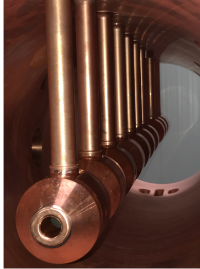
Fig 4.6: ESS DTL under assembly in Lund
