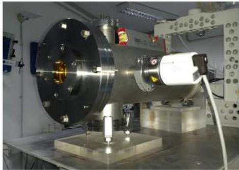
Figure 4.7: Faraday Cup mounted along the CATANA beam-line
