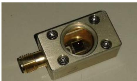
Figure 5.9: Picture of the CVD diamond detector shielded in a box
