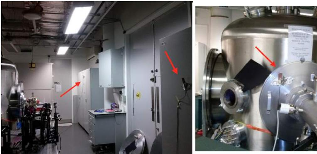
Figure 5.22: Antennas placed at different distances from the interaction-chamber at the TARANIS facility.
