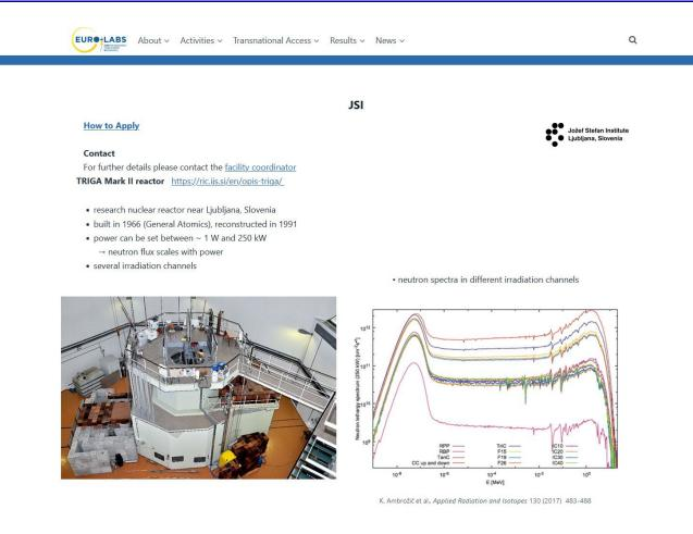
• samples are inserted to the core through vertical channels from the reactor platform
