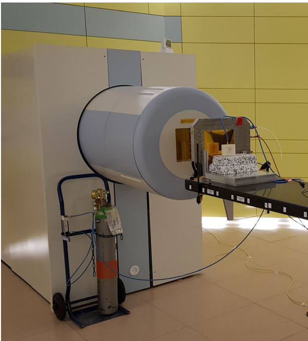
Figure 8: First commissioning for FLASH beam application at MIT using the GSI beam monitors.
