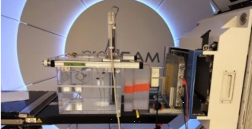
Figure 6: Setup for high-resolution dose measurement at the HollandPTC (experimental room).
