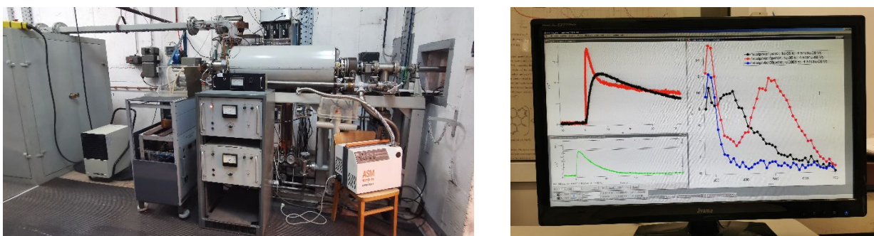
Figure 18 - View of the RAPID facility LAE 10 accelerator for nano-second pulse radiolysis experiments
