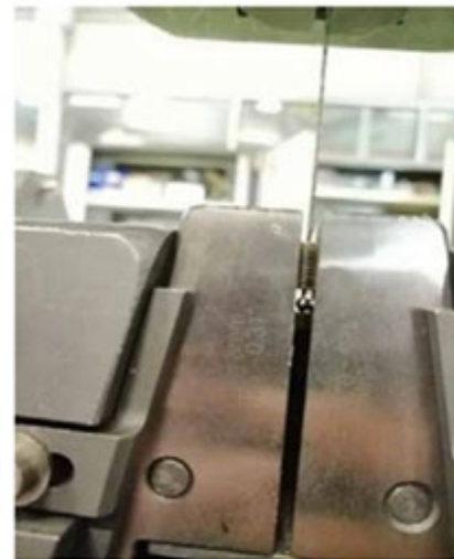
Force transfer system (welded ball and sliding tube) on the Nb, Sn strand.
