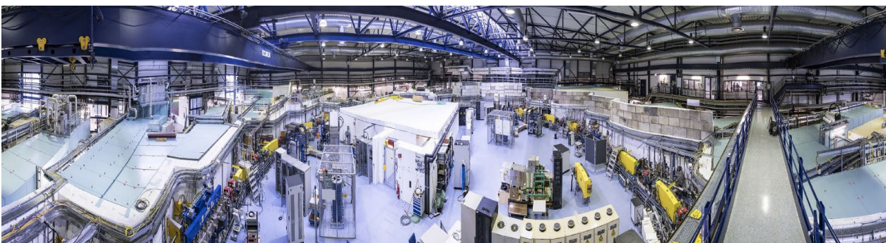
Figure 13 - Overview of the storage ring KARA, the beamlines and infra structure of the KIT Light source. KARA is part of KIT-ALFA. (Photo of M. Braig, KIT)
