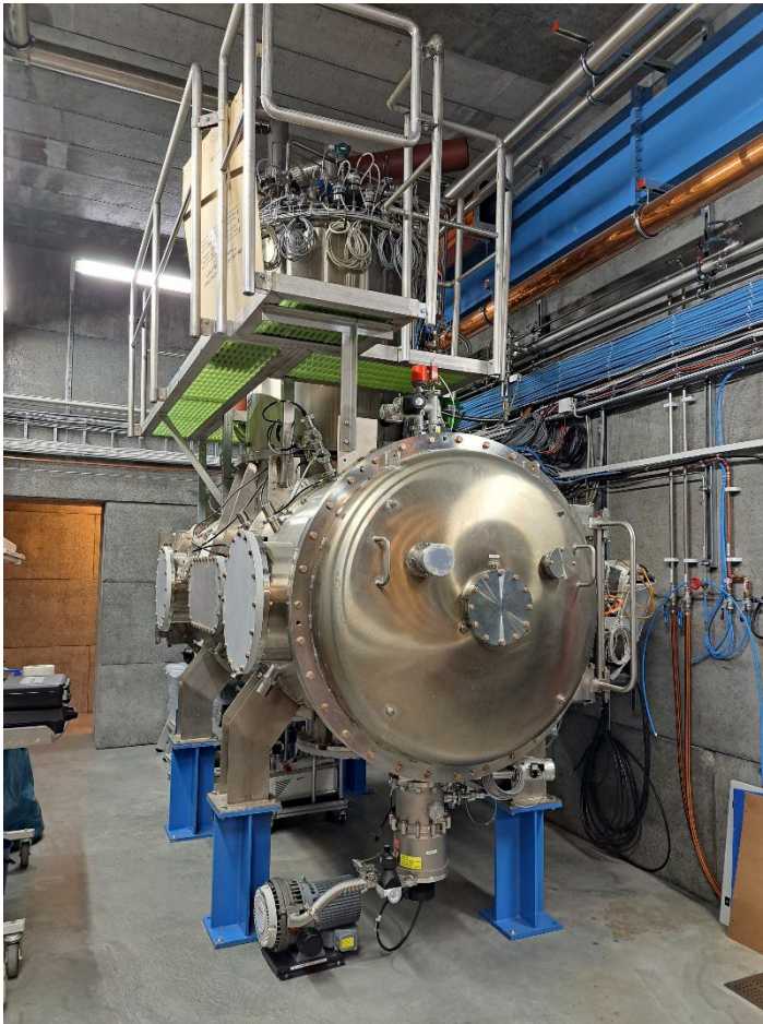
Figure 4- View of the HNOSS horizontal cryostat (left) and of the CoW portable cryostat on wheels.
