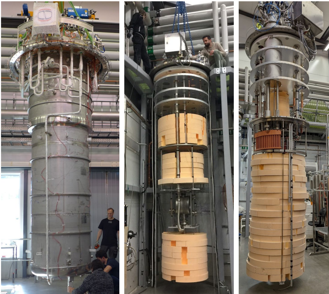
Figure 3 - View of the GERSEMI facility: vertical cryostat with pressure vessel (left), liquid insert (center) and magnet insert (right)
