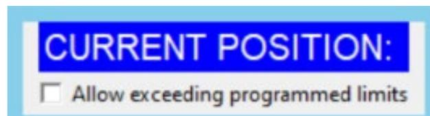
Fig. 9 Current position frame. Before homing, it displays no coordinates, because they are unknown. After homing, it displays the coordinates where the scanner should be placed according to its latest queued command.
