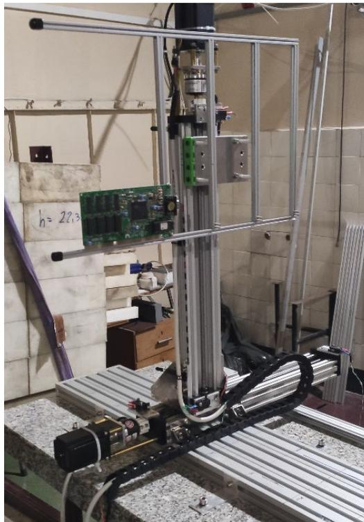
*Fig. 1 The XY table at the irradiation station at the AIC-144 at IFJ PAN. An electronic circuit mounted on the scanning surface for irradiation.*
