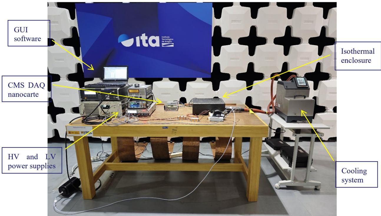
*Fig. 5 Temperature control system set-up.*
