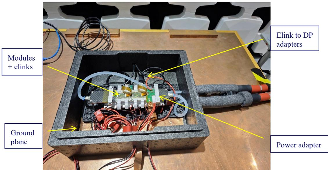
*Fig. 6 Electronics inside the isothermal enclosure.*
