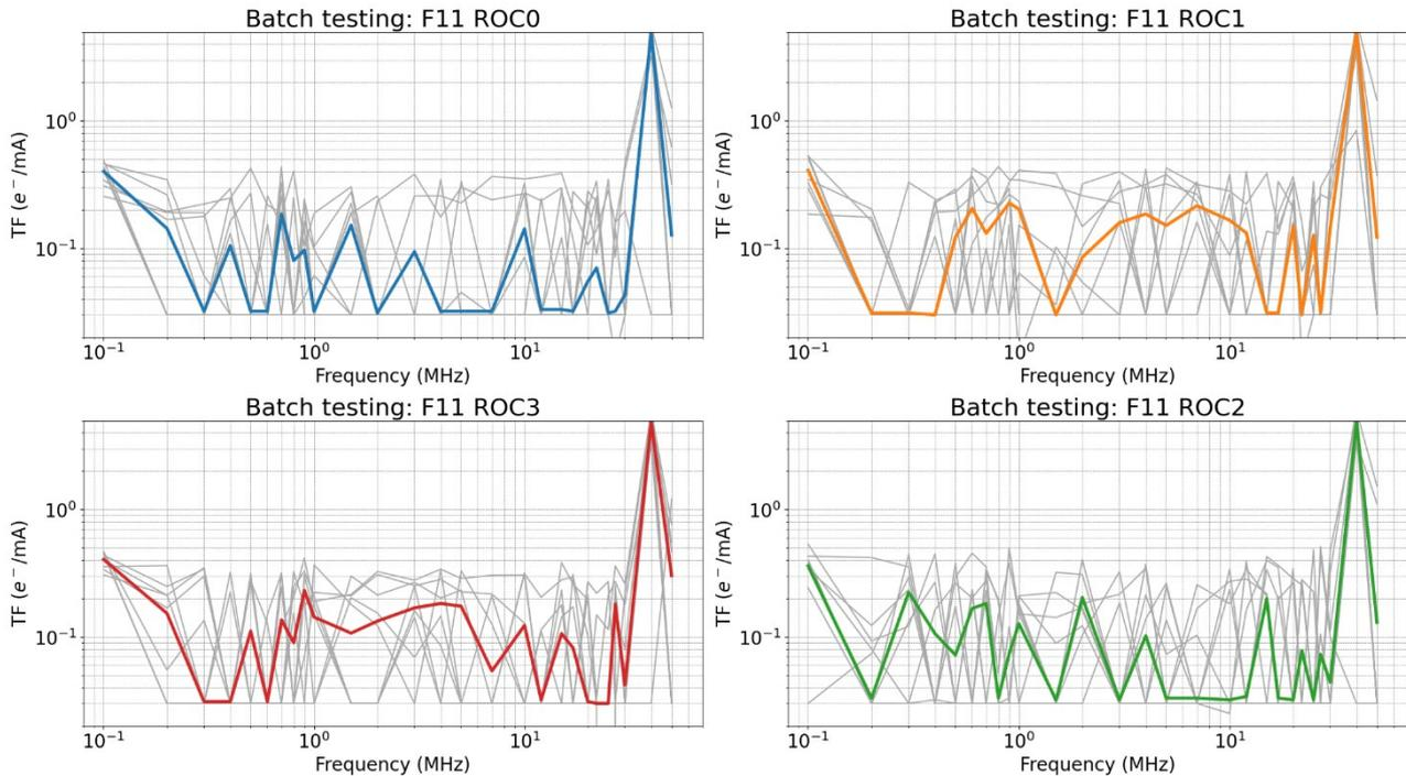
Fig. 4 Average Transfer Function (TF) of ROC0 (top left), ROC1 (top right), ROC3 (bottom left) and ROC2 (bottom right) of the module F11.
