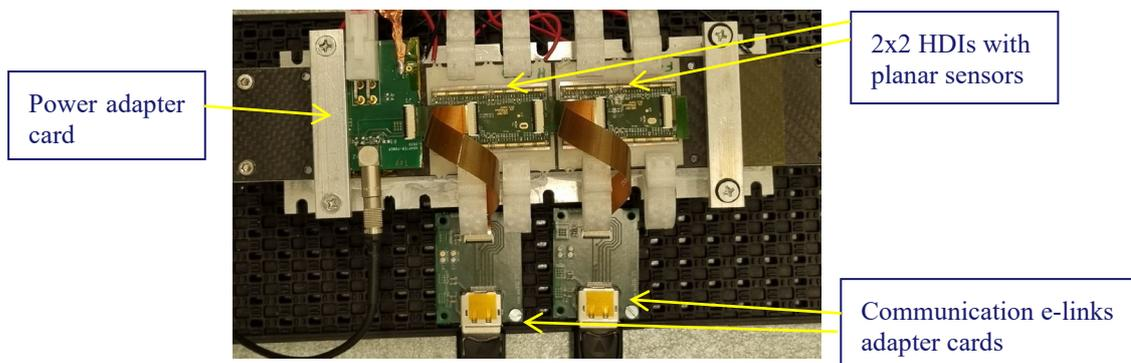
*Fig. 2 System formed by two modules in series.*
