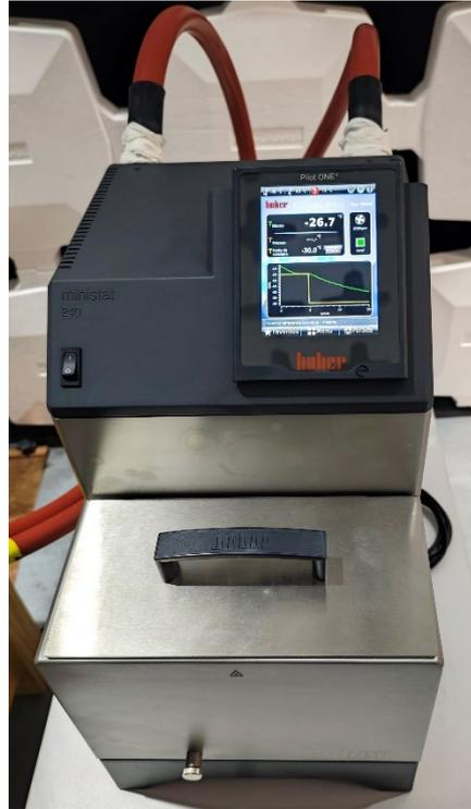
*Fig.7 Cooling system device along with the control interface.*
