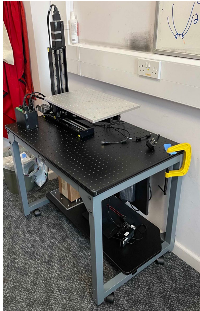
Figure 2 - The fully assembled sample scanning system. The two linear stages and sample platform are clearly visible, mounted on a portable optical table. The sample box is not present, but is easily removable from the aluminium sample platform. The control PC is also visible on the lower shelf, stored in the position ready for laboratory commissioning operations.
