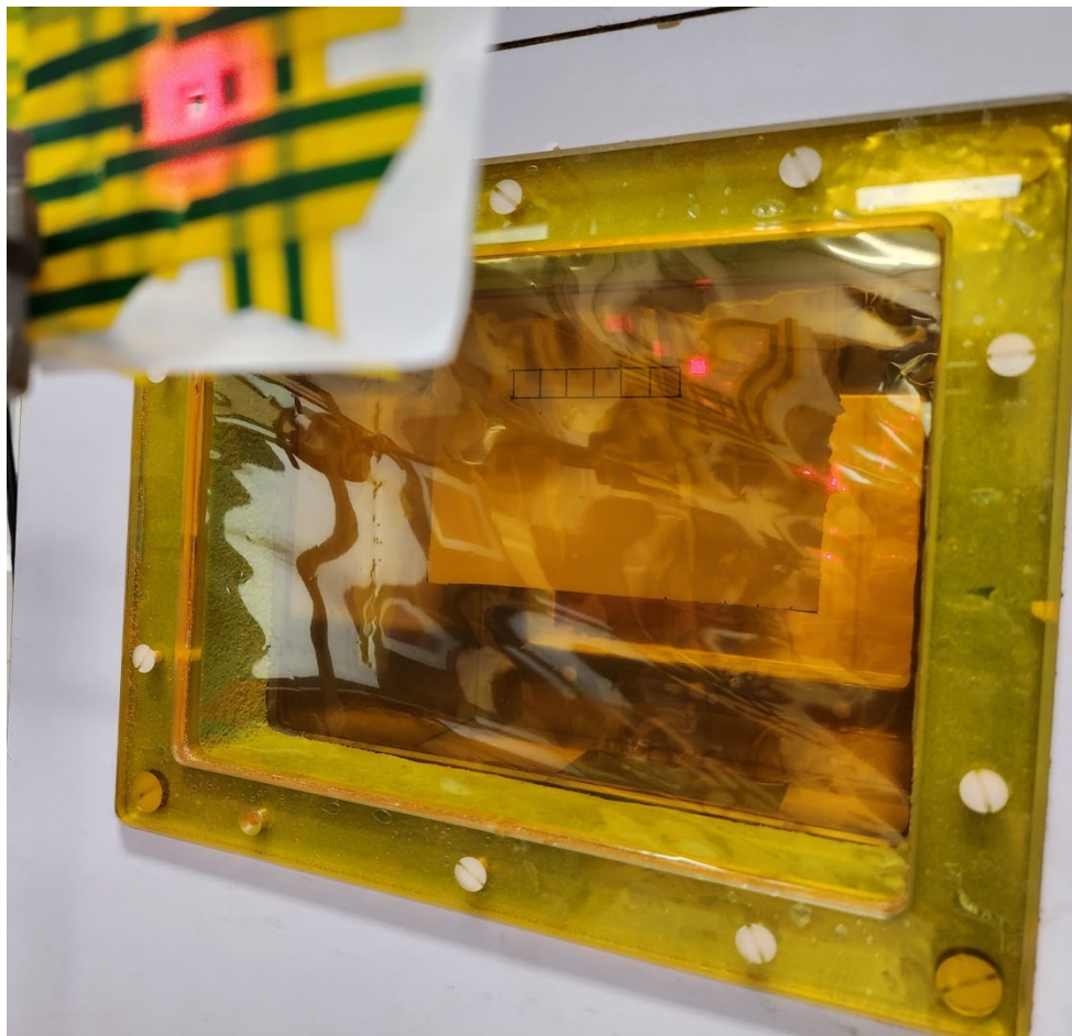
Figure 3 - The collimated laser beam entering the sample box and impinging upon the aluminium sample panel.
