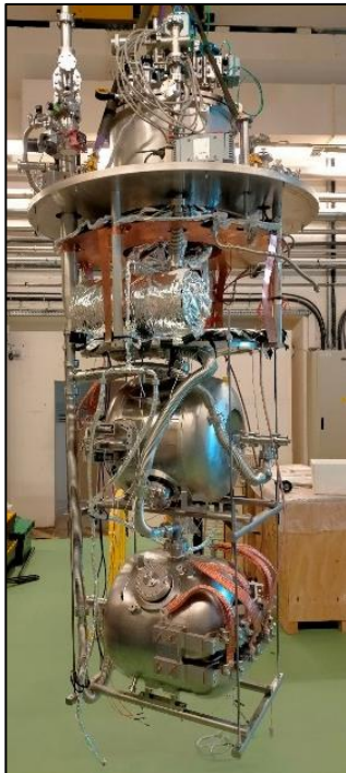
Figure 12: The test cryostat with the two prototype cavities installed.
