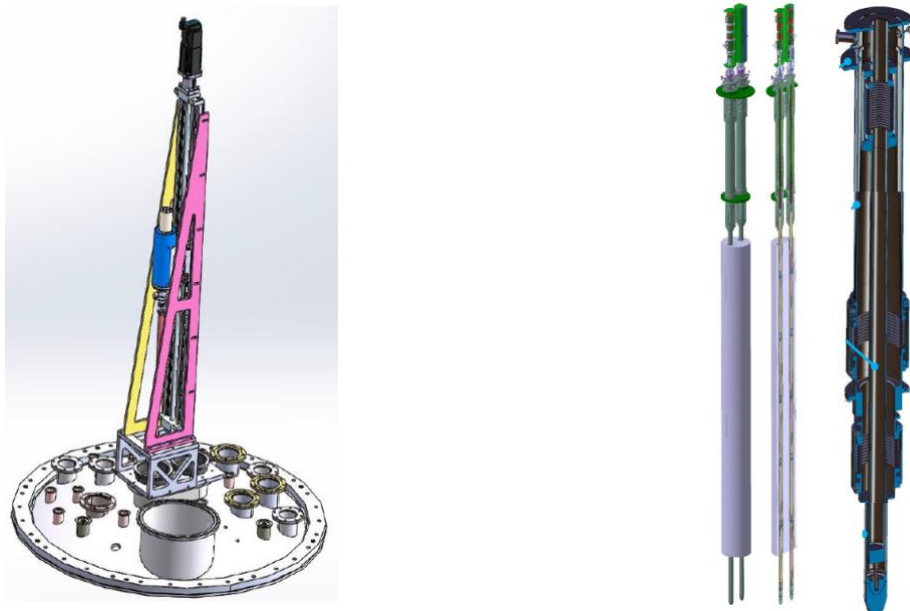
Figure 1: Schematic view of the anticryostat. Left: mounted on the cryostat flange, Right: close view of the instrumentation and the rotating coils.
