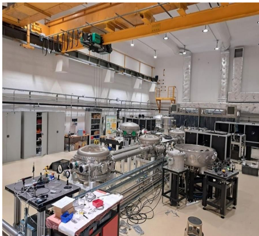
Figure 5.1: Photo of the LPA-UHI100 (Laser Plasma Accelerator on UHI100 laser facility), a platform providing an electron beam and an experimental area dedicated to laser-driven electron acceleration studies in plasma media, and applications such as FLASH Radiotherapy, secondary particles generation, diagnostic developments...etc.
