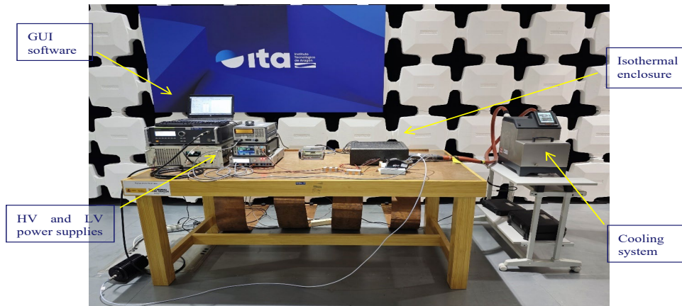
Figure 3: New TF measurement system for physics detectors (including GUI and cooling system)
