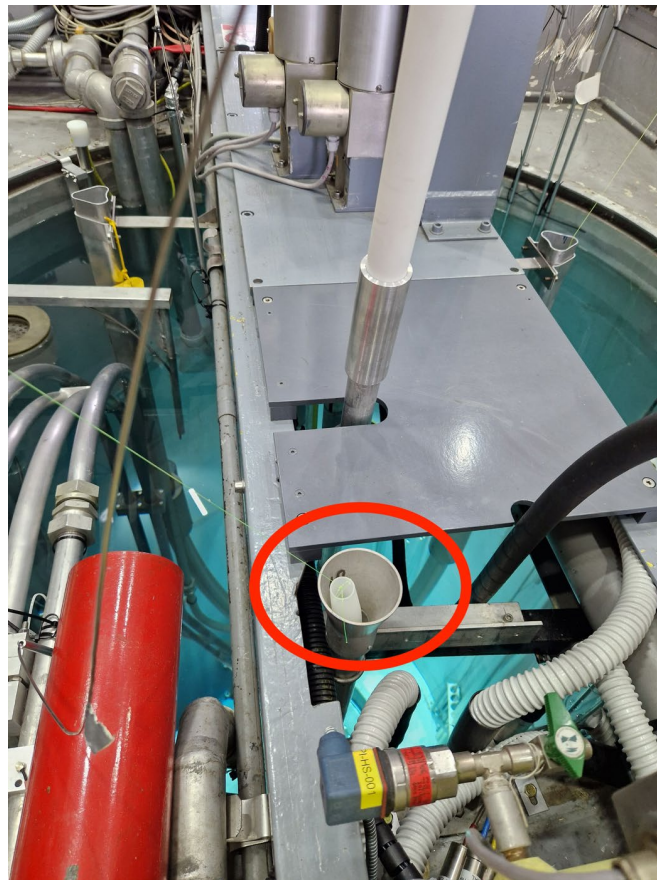
Figure 3: Insertion of samples into the F19 channel (encircled in red) leading to the reactor core faintly visible at the bottom of the water tank. The sample holder can be seen attached to the fishing rope used to lower it for irradiation and then lift it to a shielded position above the core for initial cool-down.
