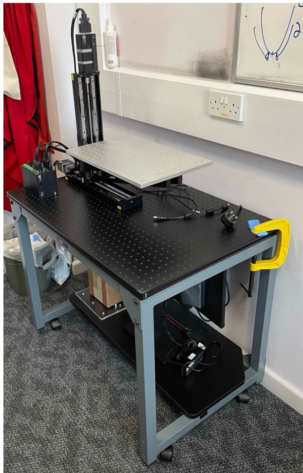
Figure 6: Upgraded sample scanning assembly during the laboratory commissioning phase.
