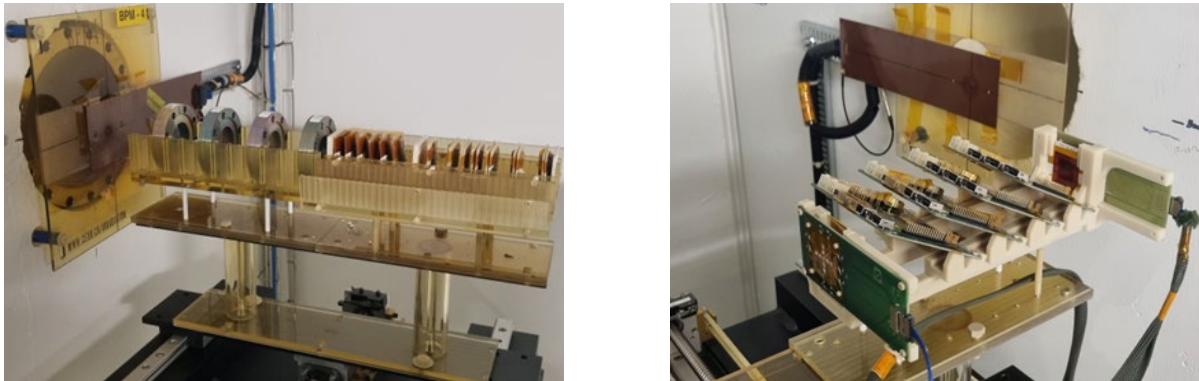
Figure 1: Examples of experiments performed during the run 2023 at the IRRAD Facility. Vacuum window samples (left-hand side) and silicon pixel modules (right-hand side).
