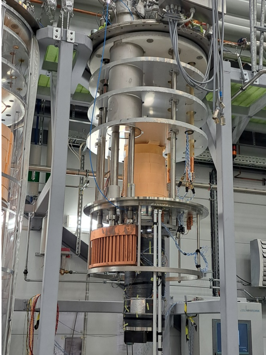
Figure 1: Picture of the CCT magnet SuShi placed on Gersemi's magnet insert.
