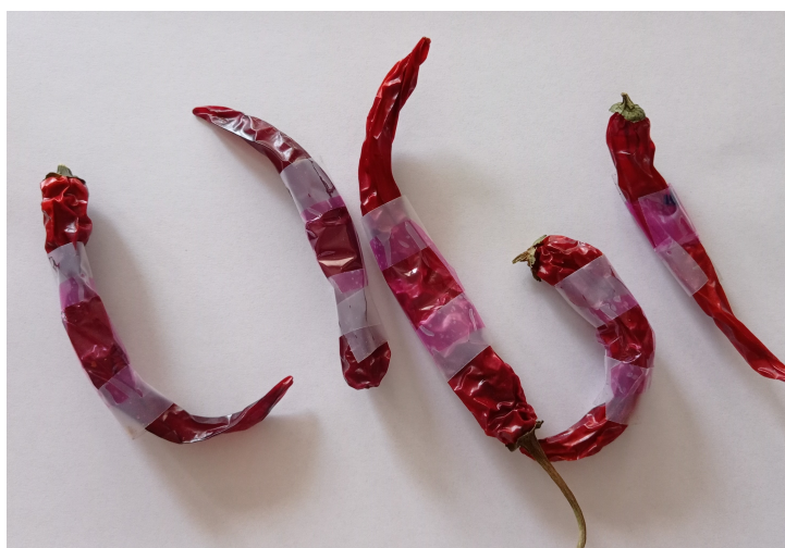
Figure 3: Chilli pepper used for dose verification for irradiation with electron beam of energy 330 keV - EURO-LABS-RAPID-2023-3
