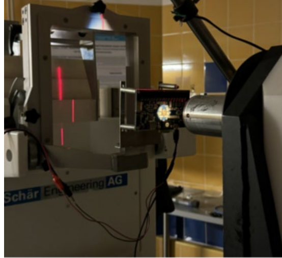
Fig. 1: Experimental setup under proton beam at the irradiation station of AIC-144
