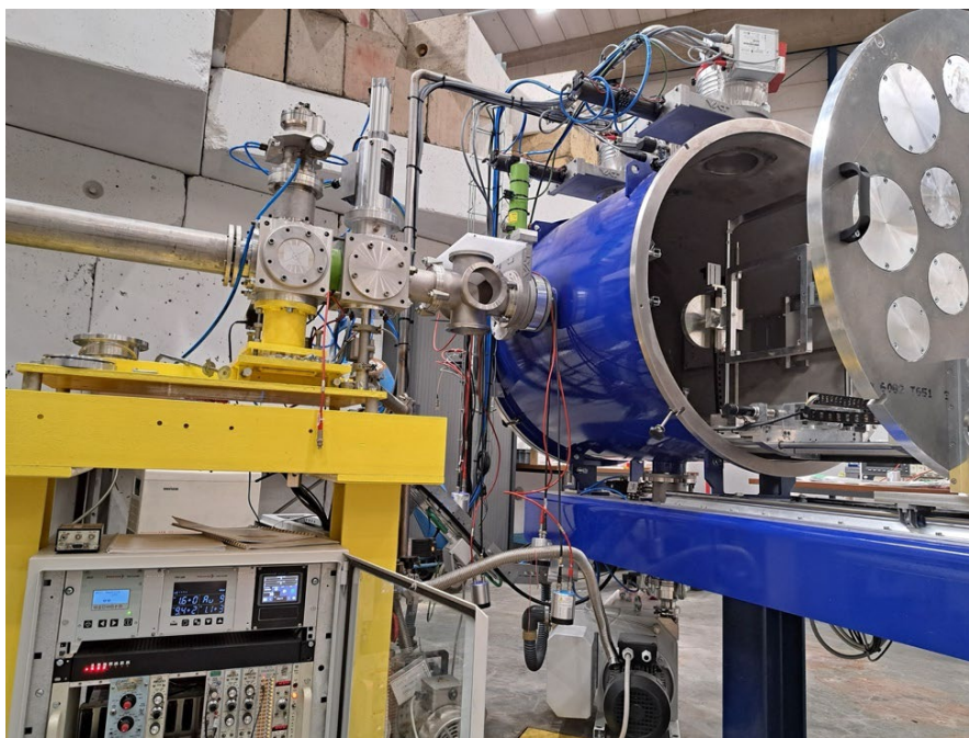
Figure 1: The end of the HIF beam line with the newly installed test chamber
