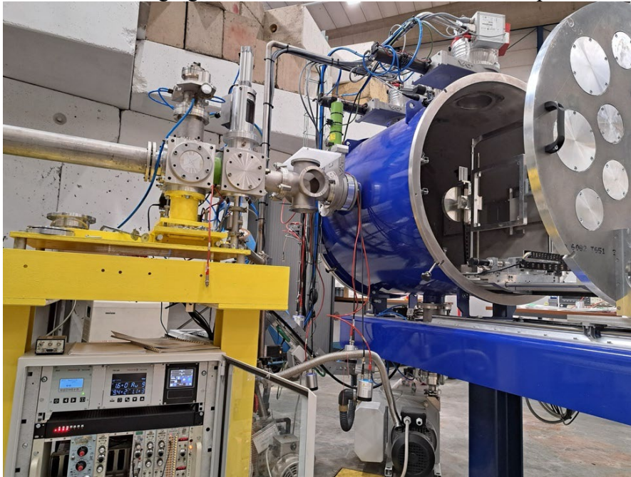
Figure 1: The end of the HIF beam line with the newly installed test chamber
