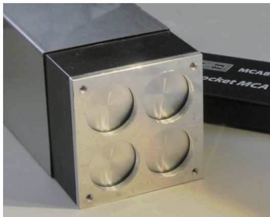
Figure 3.6: Picture of the so-called “mosaic” detection module, which is based on a 2 \times 2 matrix of \varnothing 0.5'' \times 0.5'' \text{LaBr}_3 scintillating crystals.
