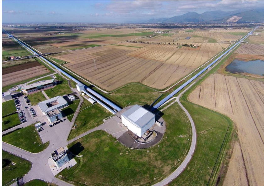
Figure 2.4. Aerial view of Advanced Virgo. The "L" shape of the detector is clearly visible here.
