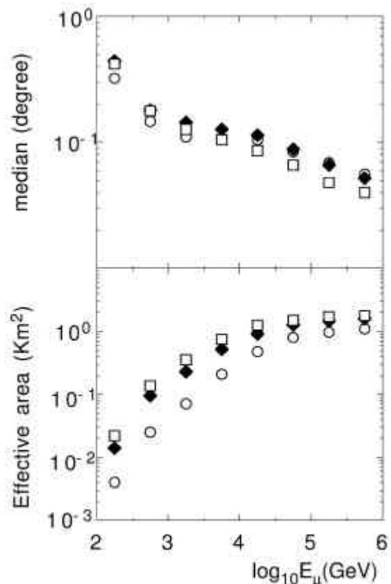
Fig. 2 – Median angles between true and reconstructed muon tracks (top) and effective areas (bottom) for 20 kHz (full diamonds) and 60kHz (open circles) after quality cuts for NEMO-dh140 detector. The open squares are the results obtained for a lattice detector with 20kHz (see text).
