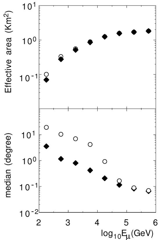
Fig. 1 – Effective areas (top) and median angles between true and reconstructed muon tracks (bottom) for 20 kHz (full diamonds) and 60kHz (open circles) for NEMO-dh140 detector.
