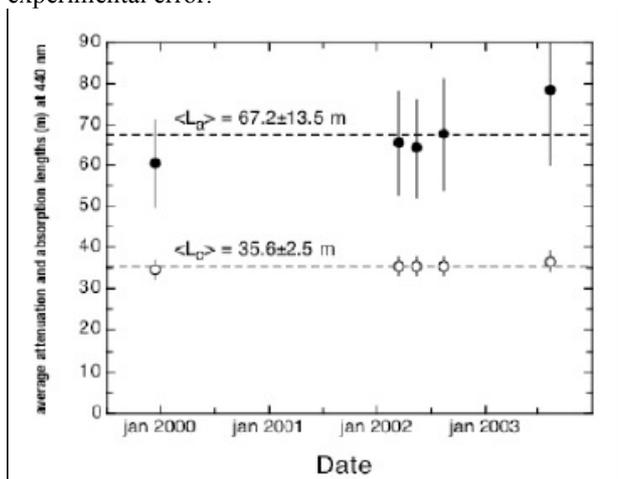
Fig. 2. Values of the absorption (full symbols) and attenuation (open symbols) lengths at 440 nm measured during five different campaigns. The reported values are the average in the depth region 2850-3250 m. Dashed lines are the average over the five campaigns.
