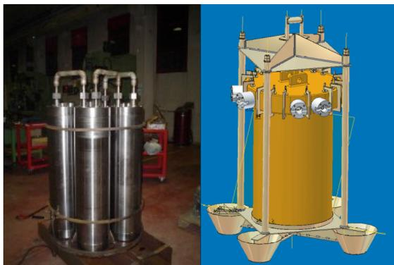
Fig. 4. The Junction Box, internal and external structure
