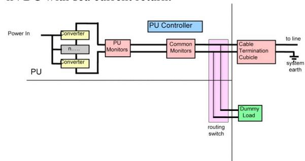
Fig. 12. Shore Power Feed Equipment
