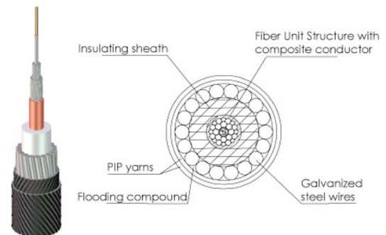
Fig. 11. Electro-optical Cable
