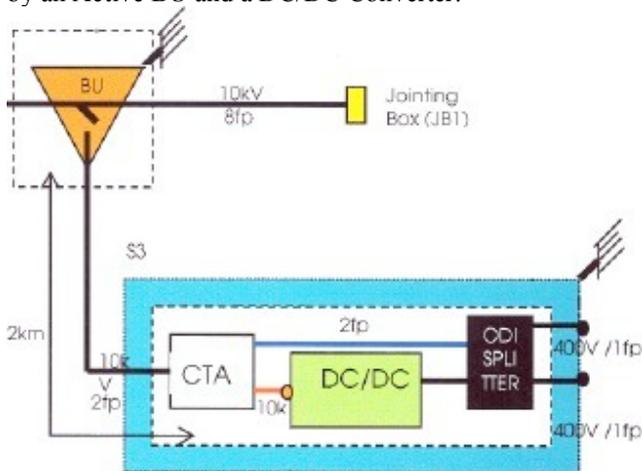
Fig. 14. Active BU and DC/DC Converter
