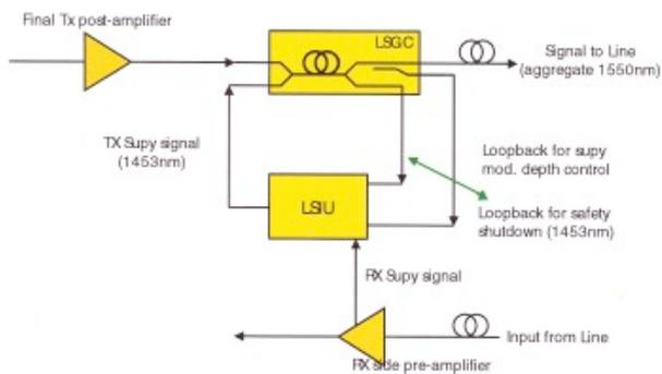
Fig. 13. Dark Fiber Monitoring Equipment
