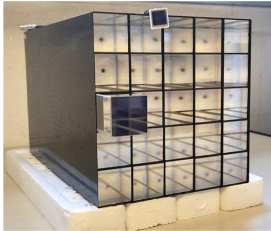
Figure 2.14: Photograph of the array of bare crystals at the heart of the MUonE ECAL with a single crystal displaced out of position for illustration purposes. One of the APD sensors used to detect the scintillation light is shown at the top of the structure.
