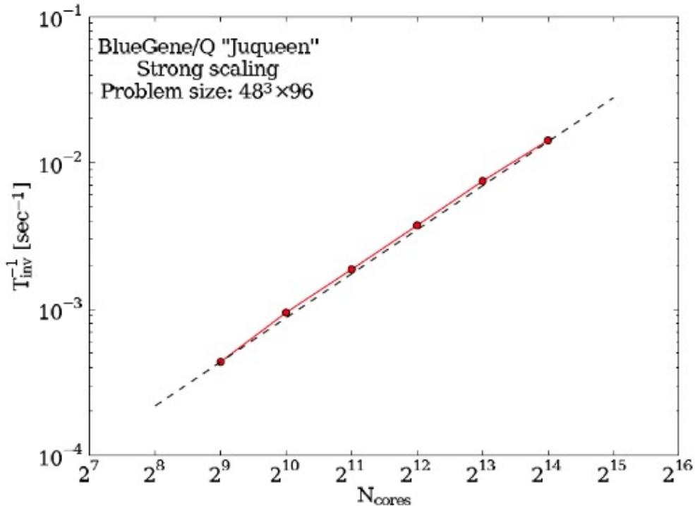
Figure 3: The inverse time to solve a problem of size  $48^3 \times 96$  on the BG/Q machine versus the number of cores used. The nice scaling behavior demonstrates that the tmLQCD package [35] can use the BG/Q machine in a massively parallelized mode.
