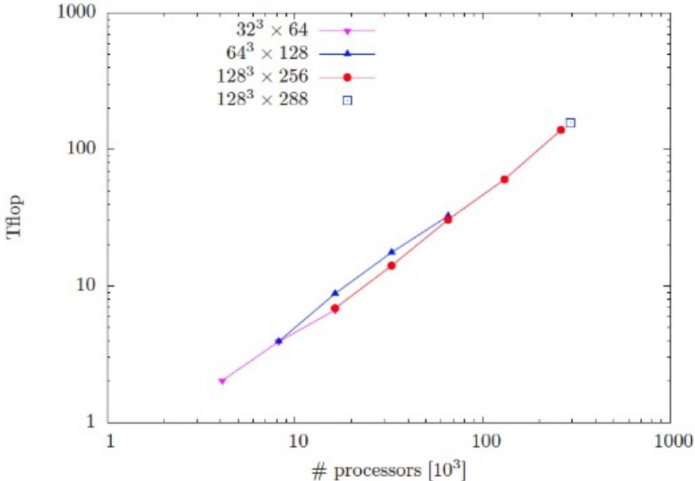
Figure 2: Performance in TFlops of the tmLQCD code [35] achieved on the BG/P versus the number of processors. The open square corresponds to the use of the full 72-rack installation at Jülich.
