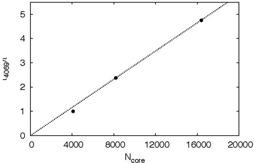
Figure 1: Scaling behavior of the MP-HMC algorithm with the number of cores on Blue-Gene/P (from [25])
