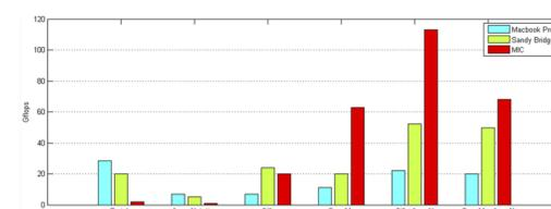
(Big) Matrix multiplications on different architectures, with different combination of array notation and OpenMP or cilk
