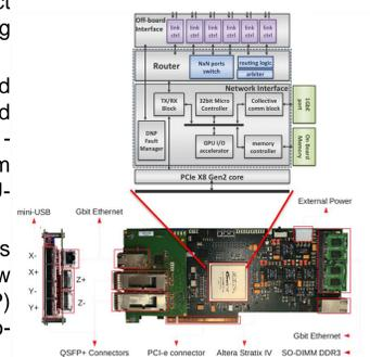
The minimization of APENet+ transfer latency is achieved through the adoption of a simple RDMA protocol implemented in FPGA with specialized hardware blocks tightly coupled with embedded microprocessor.
