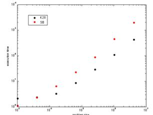
Hybrid MonteCarlo simulations of spin systems: the code is much the same for the nVidia K20 GPU (OpenACC pragmas) and for the Intel Xeon SB (OpenMP pragmas)
