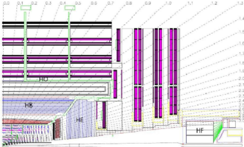
**Figure 2.8:** Schematic view of CMS where the HCAL is highlighted.
