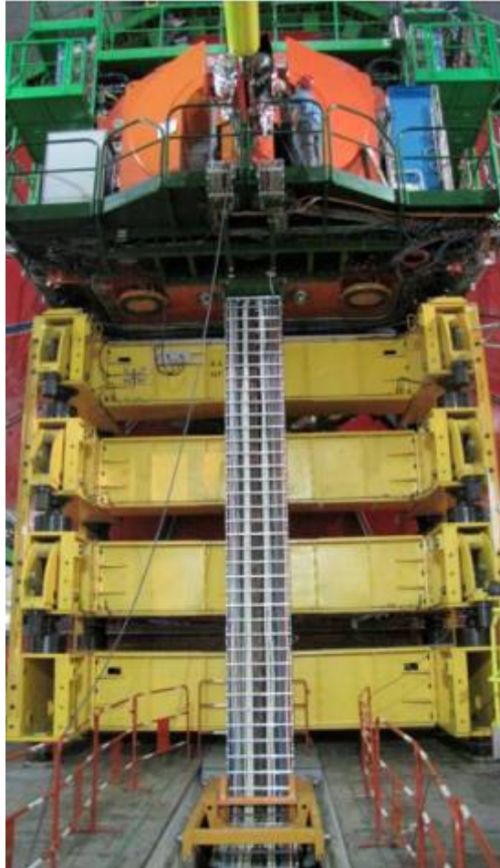
Figure 18 – Raiser (Yellow structures) supporting the Castor (Orange) and the Platform (Green) Central LHC Beam Pipe (Yellow)
