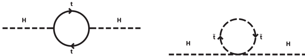
Figure 2.9: One-loop correction to the Higgs mass term from the top quark (a) and his supersymmetric partner, the stop quark (b).
