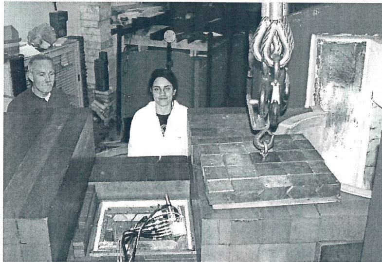
Figure 1 The Tapiro reactor thermal column. The TEPC is going to be inserted in the irradiation box, which is then closed with a graphite lid and graphite bars.
