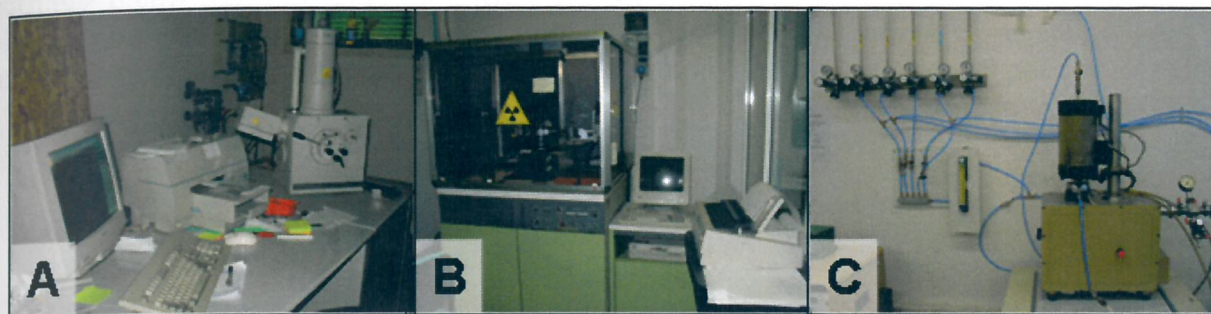
Fig. 5.10: (A) Scanning Electronic Microscope (SEM); (B) X-ray diffractometer (XRD); (C) TG/DSC thermal instrument.
