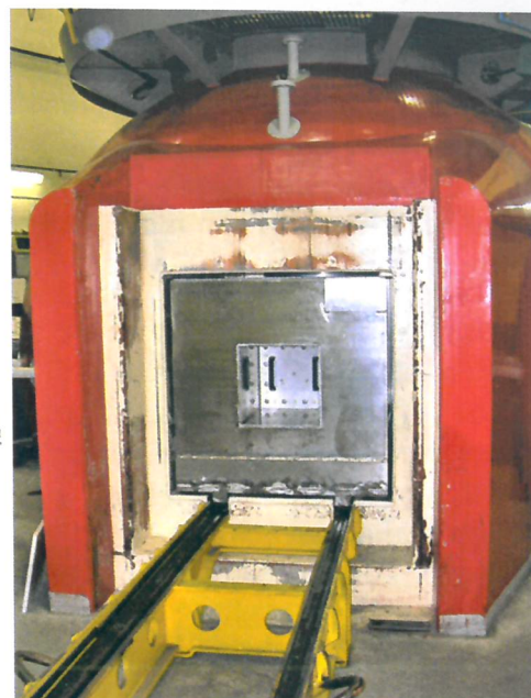
Fig. 12.26: Layout (left) and picture of HYTHOR facility. HYTHOR is 1 \times 1 \times 2 \text{ m}^3 neutron moderating structure. In the HYTHOR center, the irradiation cavity is visible.
