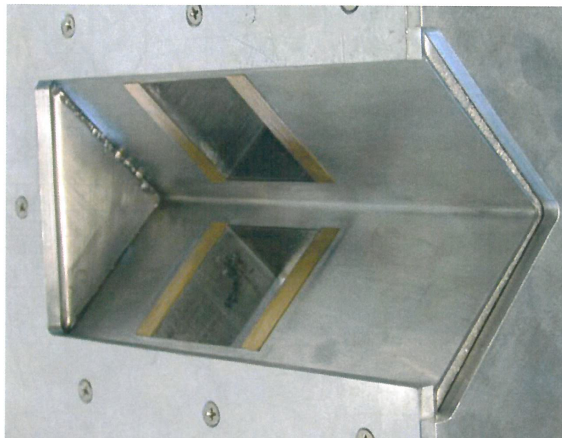
Figure 4. Bottom view of the structure, showing where the mouse is placed. Detectors face at 90°.
