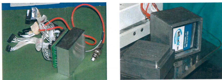
Figure 1. On the left: of integral line \text{LaBr}_3\text{:Ce} detector. On the right: picture of 10 mm \text{LaBr}_3\text{:Ce} detector with housing.
