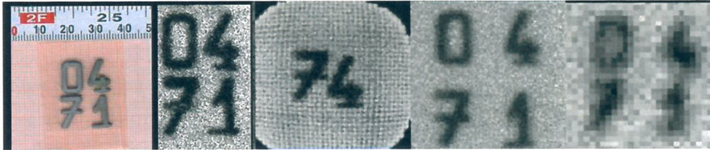
Figure 10. Lead radiological object – Absorption images. The lead mask is shown on the left. Note that the YPP imaged a mask with larger distance between the numbers in the mask.
