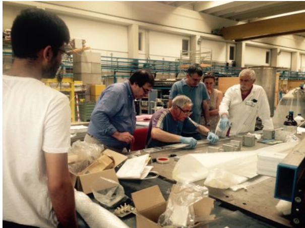
(a) Gluing I-beams, wires and gas pipes
