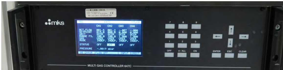
Figure 15. MKS multi gas controller 647C
