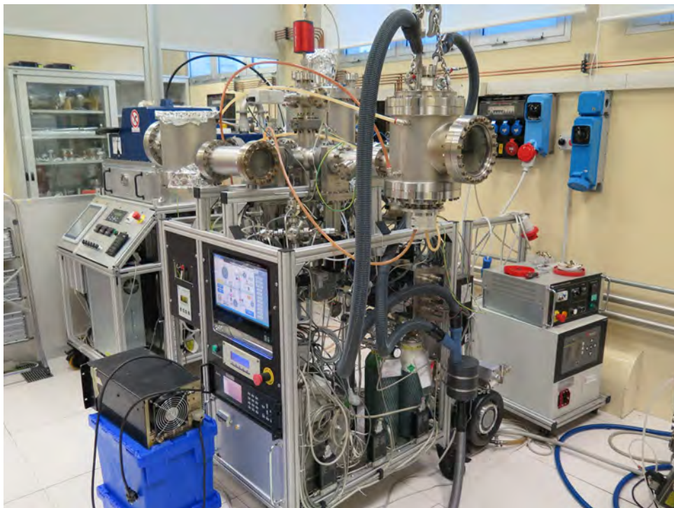
Figure 6. Upgrade of the system with aspiration ring and HEPA filter
