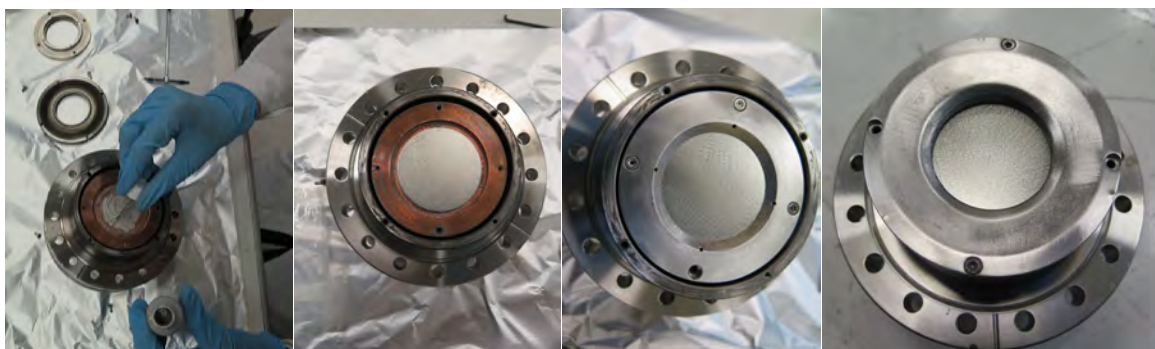
Figure 11. New Y sputtering target positioning
