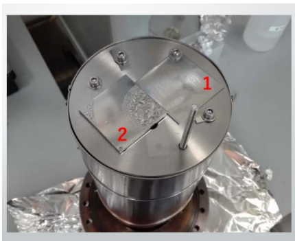
Fig. 2. The figure shows a well-done sputtering process (1) and a poorly done sputtering process (2), the difference depends on the previous polish process.
