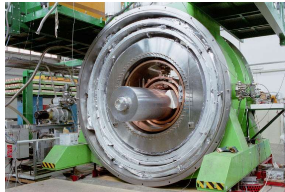
Network of 3 identical antennas : 2300 kg Al bar (3 m long, 60 cm diameter)
