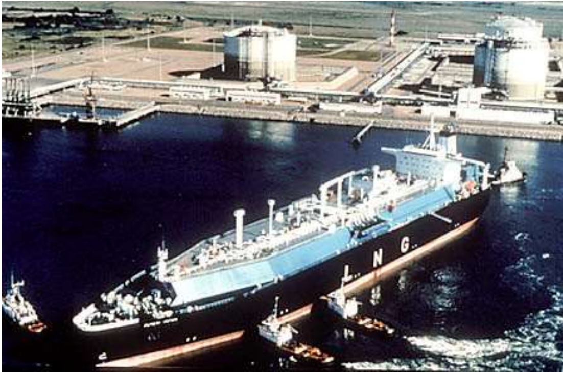
130 000 m 3 LNG carrier with integrated Invar tanks - double hull (source Gaztransport)
