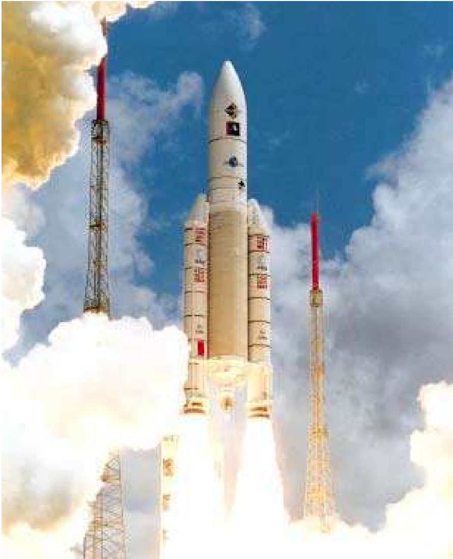
Ariane 5 (25 t liquid hydrogen, 130 t liquid oxygen)
