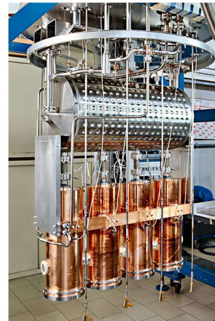
Interior of a cryostat, lodging 4 accelerating, high purity copper-based, cavities (cavity inner surface is covered by a niobium layer).
