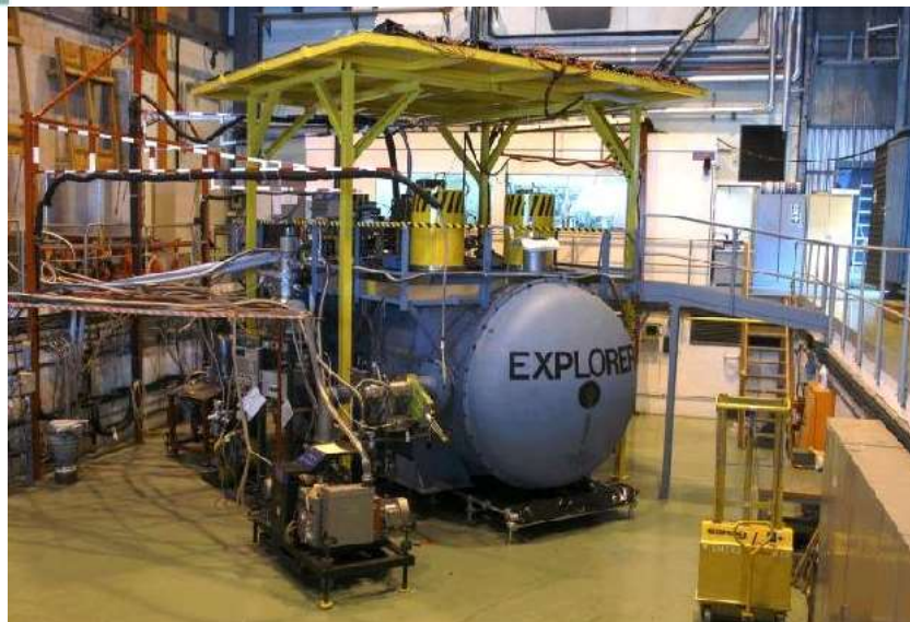
Network of 3 identical antennas : 2300 kg Al bar (3 m long, 60 cm diameter)
