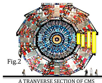
The CMS yoke is equipped with four layers of Barrel Muon Chambers named MB1, MB2, MB3, MB4 starting from the innermost ones. The 4 of a same sector are evidenced in yellow. The most exposed to the irradiation coming from the LHC interactions is the most internal layer, MB1. The diameter of CMS measures 14 m.
