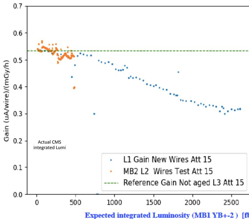
**Fig. 11** Enlarged view of the variation of gain of the New Wires of the loss of gain of the MB2 New Wires of L1 during the irradiation from Oct.2018 to Jan 2019 and , In red, the behavior of the wires of the L2 virgin layer in the short two weeks of irradiation in January.
