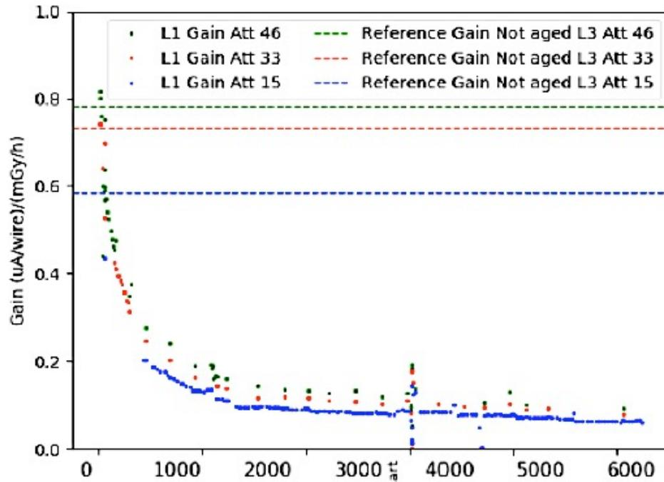
**Fig.5** The loss of gain of the MB2 chamber at GIF versus the expected integrated Luminosity (in  $\text{fb}^{-1}$ ) in HL LHC in the most exposed chambers of CMS. The total integrated Luminosity expected at the end of the HL LHC run is  $3000 \text{ fb}^{-1}$
