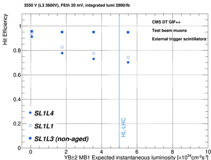
**Fig. 7** The figure shows the Hit efficiency of aged and non aged wires in function of the instantaneous luminosity measured on the GIF Muon Beam. The Muons were triggered by a set of scintillators installed along the beam line and outside the irradiation area. The tracks were reconstructed through the signals detected by the “virgin” layers of the chamber. The amplifiers threshold was set at 20 mV for all the layers.
