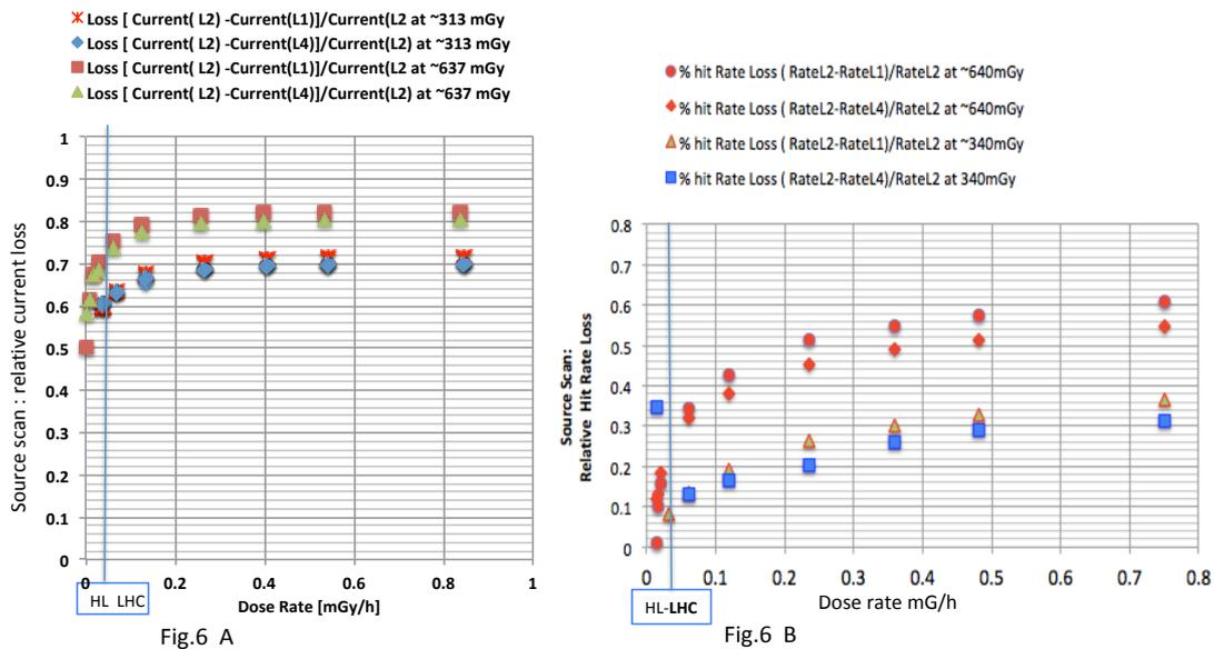
Fig A) shows that in the radiation intensity region of HL LHC the current loss of a wire after a cumulated dose of of 640 mGs ( $2300 \text{ fb}^{-1}$ ) is around 70% ,
