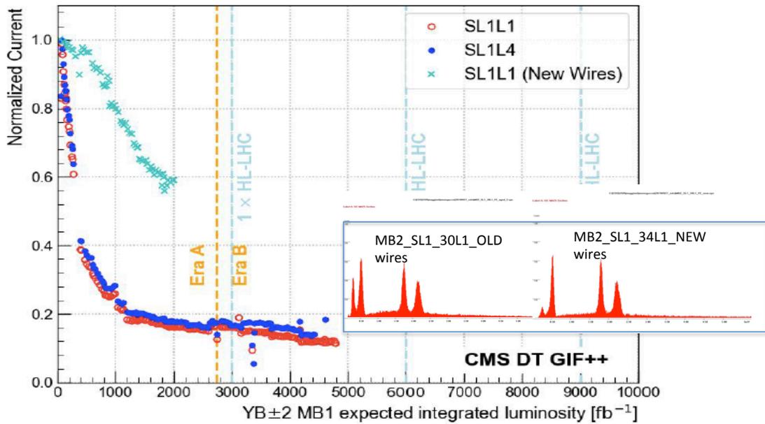
**Fig. 10** After 2000 fb<sup>-1</sup> the L1 New Wires , in green, loose 42% of the gain, the old wires loose 84%. The insert shows the eds spectra of old and New Wires (see also fig. 9)
