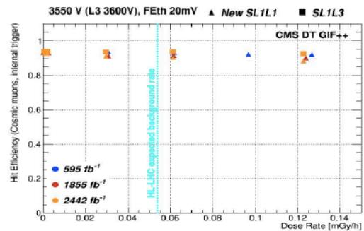
Hit efficiency for cosmic muons of the New Wires compared to the Old ones in function of the Instantaneous dose and at increasing integrated dose. The efficiency for Old and New is measured separately.
