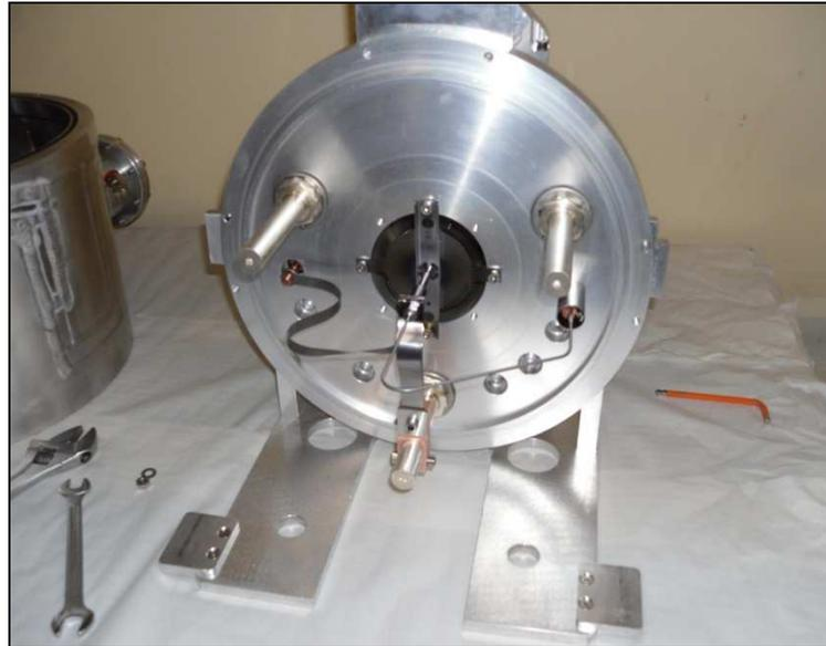
**Figure 6.8:** The SPES target chamber with the SIS ion source connects to the oven system.
