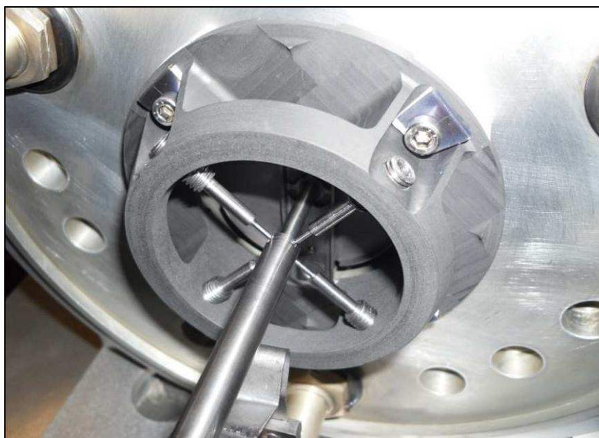
**Figure 6.7:** The SPES Positive ion source set-up (with the Ta transfer line) connected to the target-ion source chamber frame.
