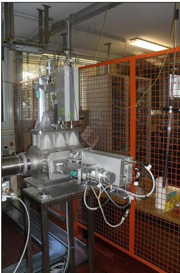
*Figure 6.6: The SPES Emittance Meter*
