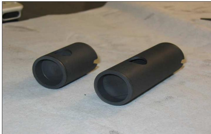
**Figure 6.16:** SiC target prototypes tested at HRIBF.
