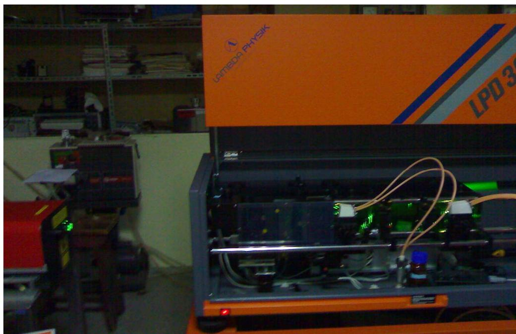
*Figure 6.15: The Pavia dye laser pumped by Nd:YAG-SHG.*
